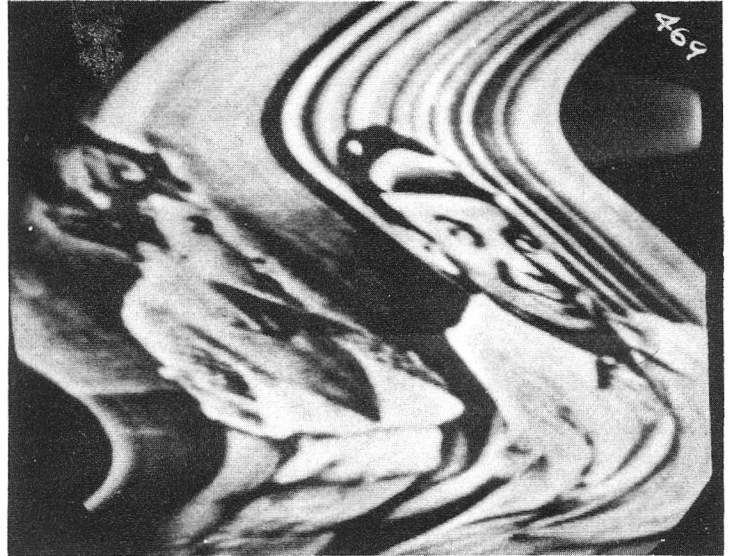
Horizontal pulling caused by heater cathode leakage in the horizontal a.f.c. circuit.
