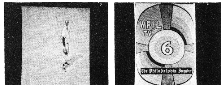
Fig. 10. Narrow picture width produced by an open linearity coil in the damper circuit of Fig. 1. This fault may affect the horizontal-output tube and the 12,000-ohm screen resistor, and result in complete absence of raster.
