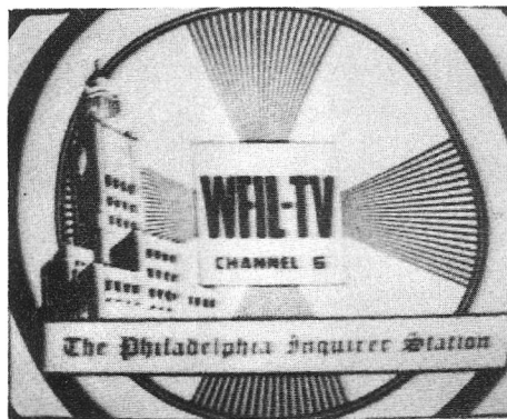
Fig. 1. Two cycles of bending between top and bottom of raster or 120 cycle change in amplitude of horizontal deflection as caused by open condensers in the "B+" filter circuit. The bending is present on the raster either with or without a picture.
