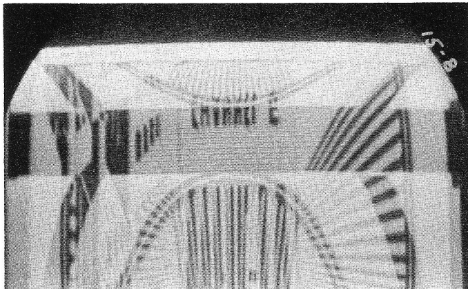
Fig. 3. When there is no vertical deflection, a quick check on the vertical output section can be made by introducing 60-cycle ac into the grid of the vertical output tube. When this picture was made the coupling capacitor between the vertical oscillator and the vertical output tubes was opened, and 60-cycle voltage was introduced into the grid of the output tube by placing a finger on the grid. The hum voltage picked up by the body is usually sufficient to produce some vertical deflection as shown above. Note in this picture that the test pattern appears to be wrapped around a cylinder, due to the sine-wave deflection. This simple check shows that the vertical output circuit, including the tube, output transformer, and vertical deflection coils, are in operating condition, thereby indicating that the trouble is ahead of the vertical output tube. As mentioned previously, the fault in this case was an open coupling capacitor between the vertical oscillator and output tubes. This system of "signal injection" to find troubles quickly in the vertical deflection circuit can be extended and improved by using a good audio oscillator, such as the RCA WA-54A to provide a 60-cycle sine-wave signal of adjustable amplitude. First feed the audio oscillator directly across the vertical deflection coils, then across the primary of the vertical output transformer, then into the grid circuit of the vertical output tube, and finally into the output circuit of the vertical oscillator. Absence of vertical deflection on the kinescope at any one of these test points will reveal the location of the trouble.
