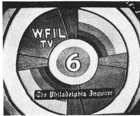
detected by observing vertical sync on the tube, as shown in Fig. 9. The fault here is the incorrect setting of the a.g.c. threshold adjustment, permitting excessive signal input to video amplifier, where the limiting action reduces the amplitude of the sync signals.
