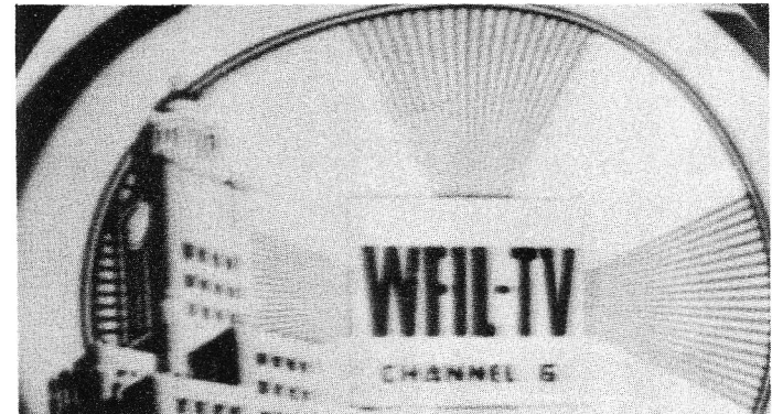
Fig. 10—Picture stretched at left produced by open resistor across damper tube
