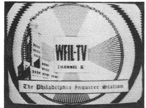
wedges is one indication of regeneration in amplifier which requires realignment. Regeneration in this case results from tuning grid and plate circuit of one stage in amplifier to same frequency instead of staggering tuning as required in stagger-tuned amplifier.
