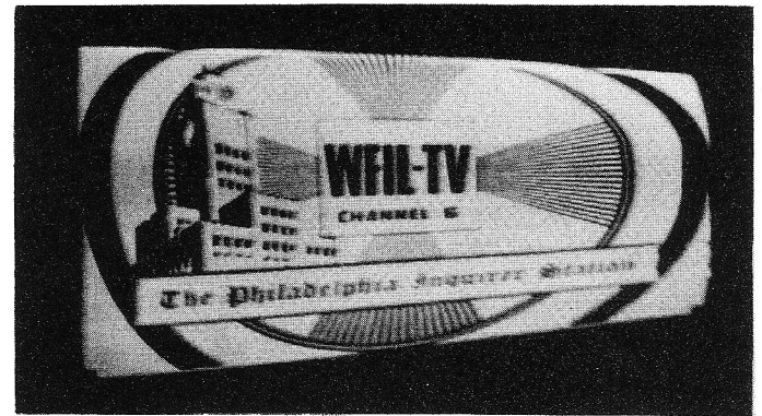
Fig. 5. Same effect as in Fig. 4, but the other half of the vertical deflection coil is shorted, causing keystone in the opposite direction.
