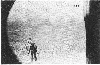
Fig. 7. Same condition as in Fig. 6, except that the position of the hum symptoms has been shifted by reversing the power-cord plug.
