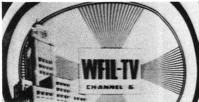
Fig. 6—Bright vertical line at right, and picture expanded at left produced when the 0.035-uf capacitor in plate return of horizontal output tube is opened; drive control set full clockwise.
